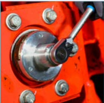
Operating using ratchet with inserted 12.5 mm (1/2") 4-point socket
