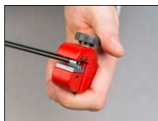
Positioning of line to scrape the covering
