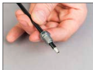
Mounting the union nut
